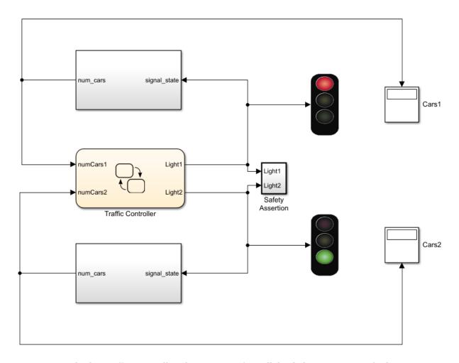
Inside the Traffic Controller chart, a pair of parallel subcharts manages the logic controlling the traffic lights. The subcharts have an identical hierarchy consisting of three child states: Red, Yellow, and Green. The output data Light1 and Light2 correspond to the active child states in the subcharts. These signals:
