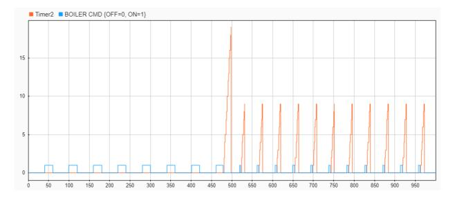
The shorter cycle and longer cooling time are a consequence of the substate hierarchy inside the On state. When the boiler reaches the reference temperature for the first time, the transition from HIGH to NORM keeps the controller on for an extra time step, resulting
